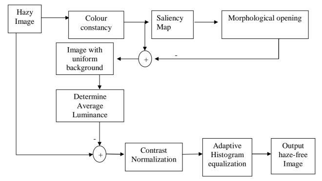
Fig. 1.Schematic representation of the proposed method
